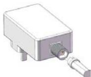
Plug attachment: Firmly attach the plug (supplied separately) to the unit's power cord by screwing it onto the screw-threaded attachment at the end of the cord – see diagram.
