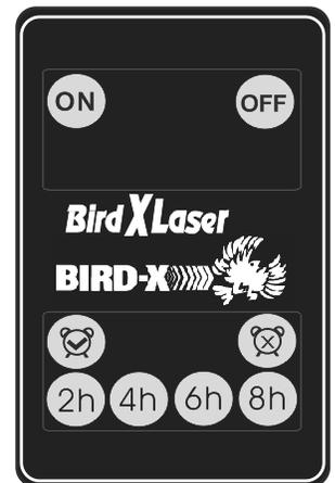
To use the timer, press the remote’s TIMER ON button. Unit will flash twice to show it has received the signal. Pressing the TIMER ON button defaults to 2 hours of operation. To select a different duration, press the desired hour button following Timer START. To cancel timer operation, press the TIMER OFF button. Unit will flash twice to show it has accepted the signal.
